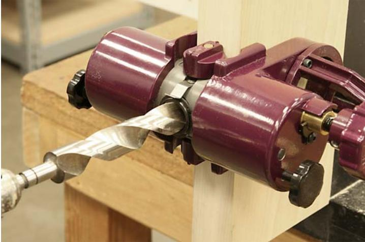
We are using a 1 inch brad point bit for drilling the edge bore. Again use a low RPM and back out the bit to help remove chips.
