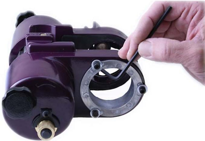
Using the supplied allen wrench, install the proper size break out plate/hole saw guide. Two 1-1/2" and two 2-1/8" guides are supplied. For wood door use mount with the washers on top of the break out plate. For steel door use, mount with the washers under the break out plate. Remove the multi-spur guide on opposite side and replace with another guide as shown in picture.
