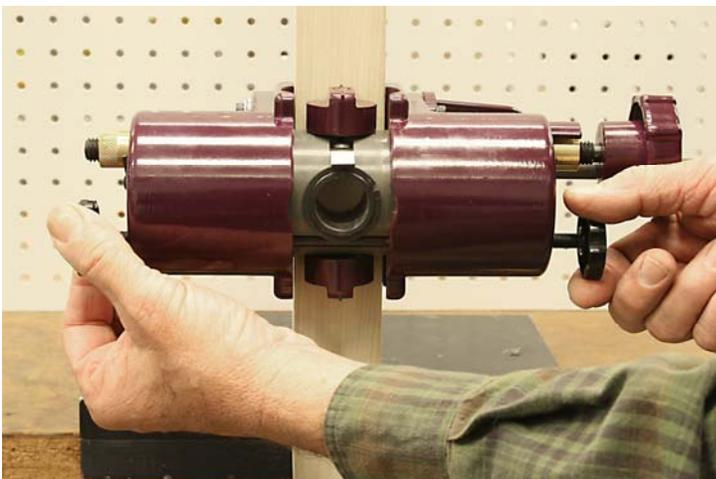
Now tighten the black plastic cantilever knobs until snug.
