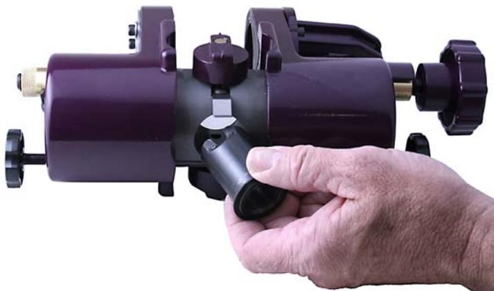
There are three drill guide bushings supplied with the HIT-44 for use when drilling the edge bore, they are held in with a clip. Choose from a 7/8", 1" or the brass guide for use with a multi-spur bit, they just snap in.
